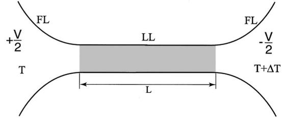
FIG. 1. Schematic of a Luttinger liquid (LL) nanowire of length  $L$  connected to Fermi liquid (FL) reservoirs kept at different temperatures and bias voltages.
